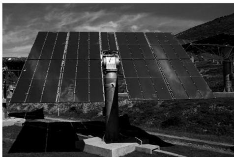
图2 玻璃反射镜 Fig.2 Faceted glass heliostat
