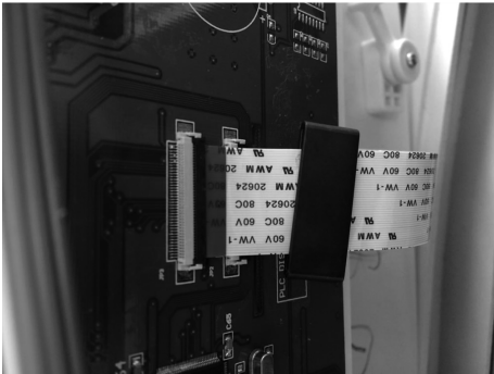
图8 针对排线的整改措施 Fig.8 Corrective measures for ribbon cable
