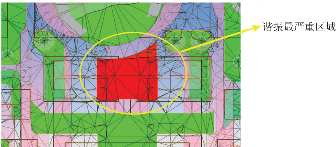
图 11 谐振最严重处细节图 Fig. 11 Details of the most severe resonance
