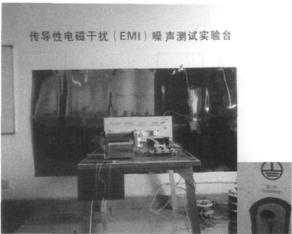
图 5 实际传导性噪声干扰测试实验场地(接地面与大地连接) Fig.5 The actual test setup of EMI(connection between the ground and the earth)
