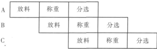
图 1 工序流程图 Fig.1 Working procedure flow chart
