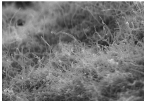
图 5 经过水浴处理后的阴极表面碳纳米管分布 Fig.5 SEM picture of CNTs morphology after bathing process
