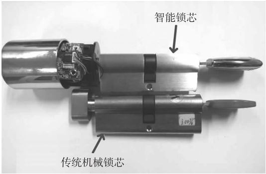
图 5 智能锁芯和普通机械锁芯的实物对比如照片 Fig.5 Photograph of the smart lock cylinder and the traditional mechanical lock cylinder
