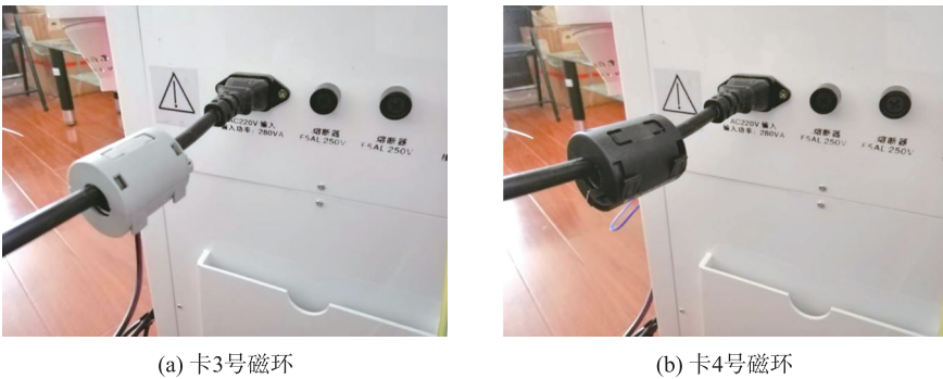
图 15 在臭氧机的电源线上卡扣材料不同的磁环 Fig. 15 The power cord of the ozone generator is buckled with only magnetic rings with different materials.
