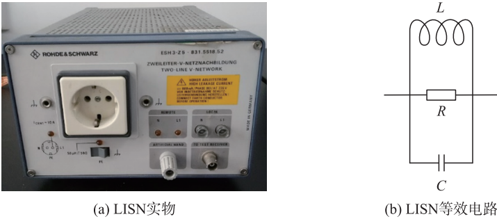
图 4 LISN 及其等效电路 Fig. 4 LISN and its equivalent circuit
